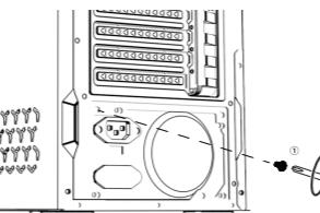
Please make sure that the holes of power supply aim at case cooling vents when installing power supply.
