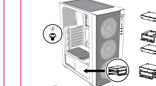
Hard disk enclosure for both SSD and HDD; unscrew hard disk enclosure and install HDD with screws.
